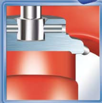
Diverse materials acc. to application e.g. stainless steel option (machined seat)
